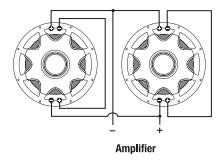
Series-Parallel wiring two dual 2 ohm subs = 8 ohm
