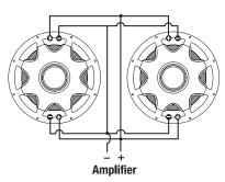
Parallel-Parallel wiring two dual 2 ohm subs = 1/2 ohm
